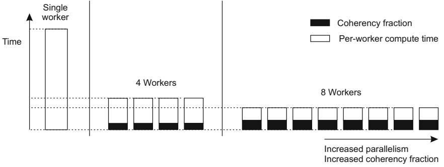
Fig. 2. The effect of coherency delays on speedup.
