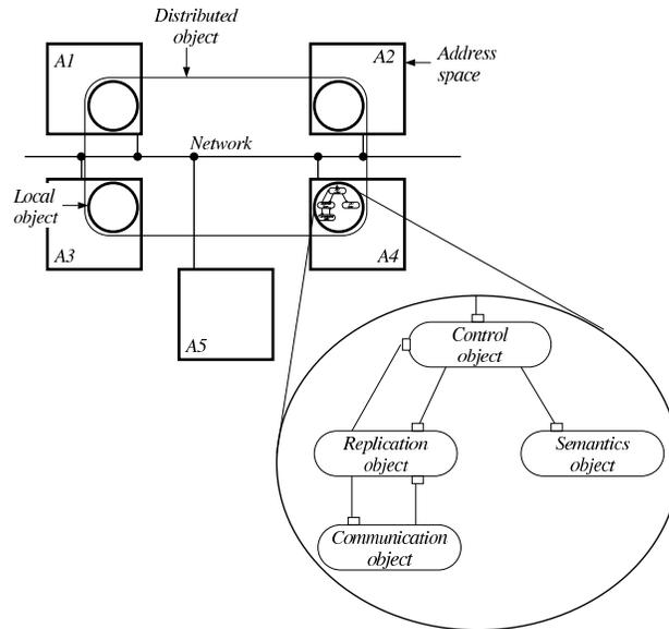
Figure 1: The structure of a Distributed Shared Object.
