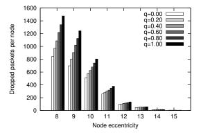
Figure 8: Dropped packets for p=0.60 and message generation rate 20 msg/sec, for different values of compensation probability q. Only nodes with eccentricity 8 or 9 apply this probability q for transmitting in the compensation phase. Note that q=0 corresponds to probabilistic flooding whereas q=1 corresponds to the original GOSSIP3.
