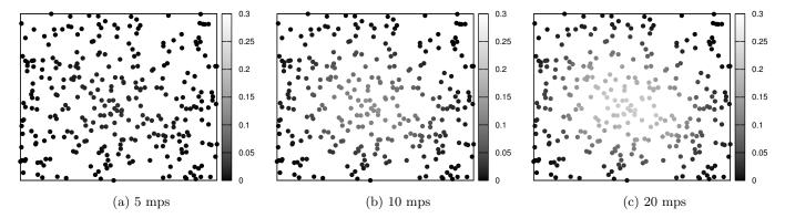
Figure 4: Packet drop rate per node for p = 0.60 represented by the intensity of the dots. As the frequency of message generation increases, so does the number of dropped packets for central nodes.
