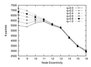
Figure 7: Number of rebroadcasts per node for p = 60 and message generation rate 20 msg/sec. Lines plot different values of compensation probability q.
