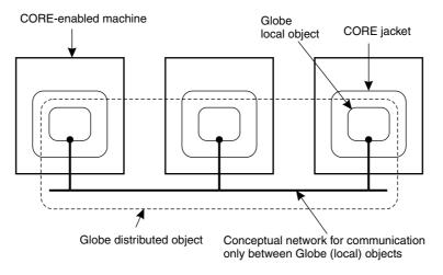
Fig. 5. The integration of remote and distributed shared objects into a single model.
