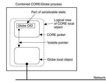
Fig. 6. The relation between a jacket and its associated Globe local object.
