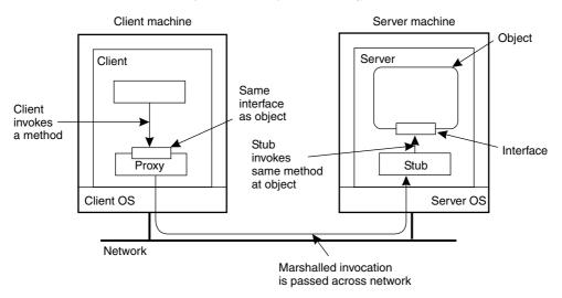
Fig. 1. The principle of a remote object.
