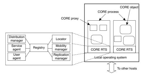
Fig. 2. The organization of a CORE-enabled host.
